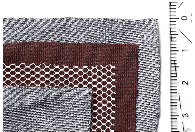
Fig. 1. The 4 fabric layers, as embedded in the flexible tactile sensor. A piezoresistive fabric and honeycomb mesh are located between the two highly conductive electrode layers.
